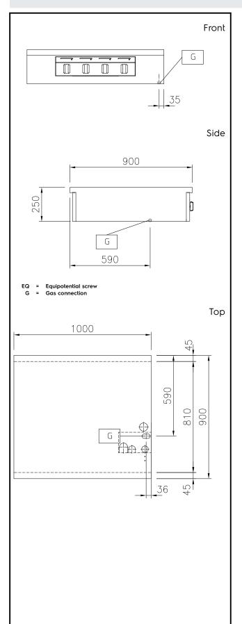
Gas Gas Power: 34 kW Gas Type Option: Gas Inlet: 1/2" **Key Information:** External dimensions, Width: 1000 mm 900 mm External dimensions, Depth: External dimensions, Height: 250 mm Net weight: 82 kg Configuration: One-Side Operated;Top Front Burners Power: 8.5 - 8.5 kW **Back Burners Power:** 8.5 - 8.5 kW **Back Burners Dimension -**Ø 70 Ø 70 Front Burners Dimension -
